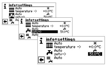
Set the required domestic hot water temperature (= setpoint value): 30 °C. Terminate input. This saves the required temperature.
