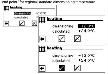
The program of the heating and heat pump regulator now calculates the actual return temperature at -12 °C for the heating curve end point and displays this in the menu field "Calculated". In the example+24,0 °C:
